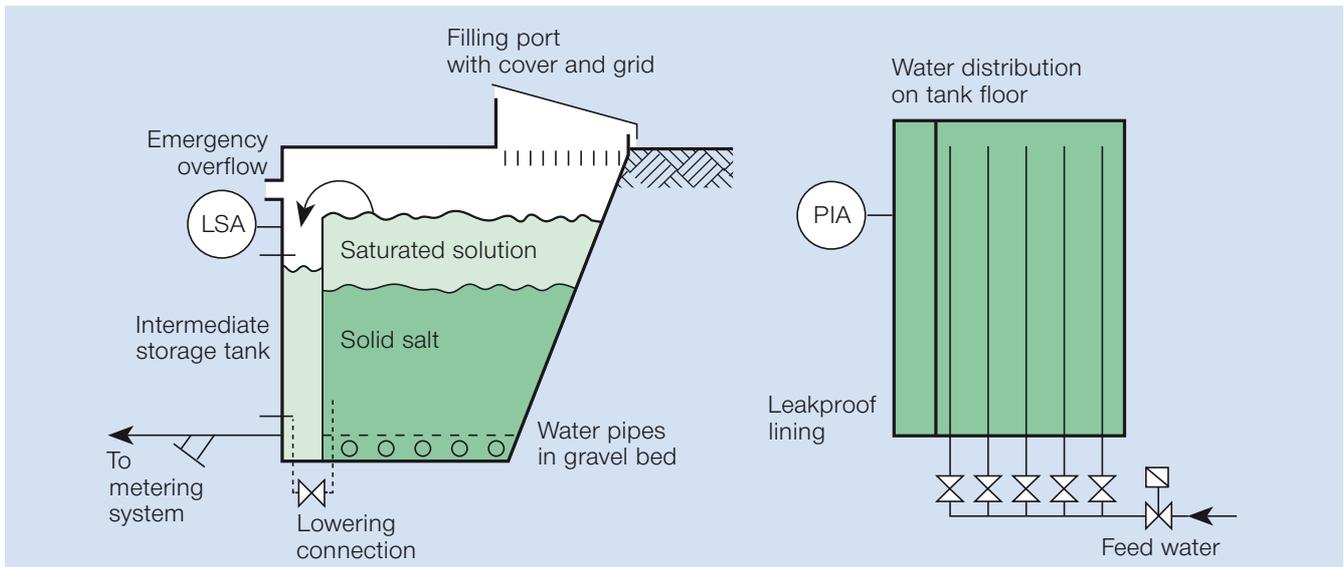
Figure 2: Diagram of a storage and dissolution installation (soaking tank) for salts
