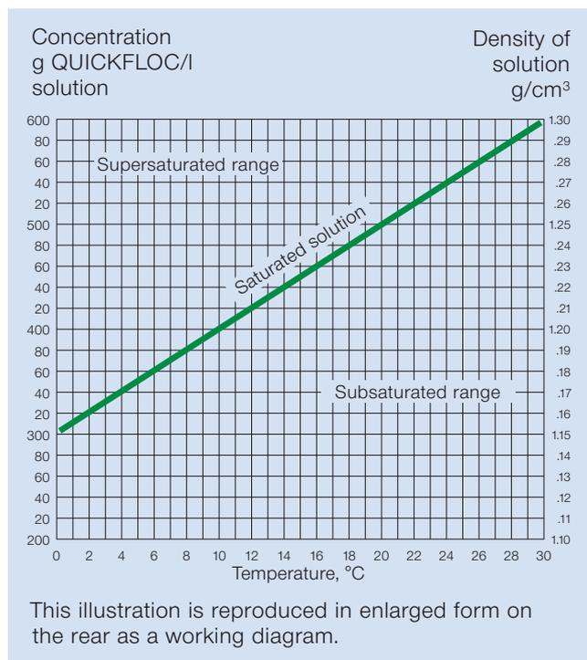
Figure 1: Solubility and density of QUICKFLOC ferrous sulfate in water
