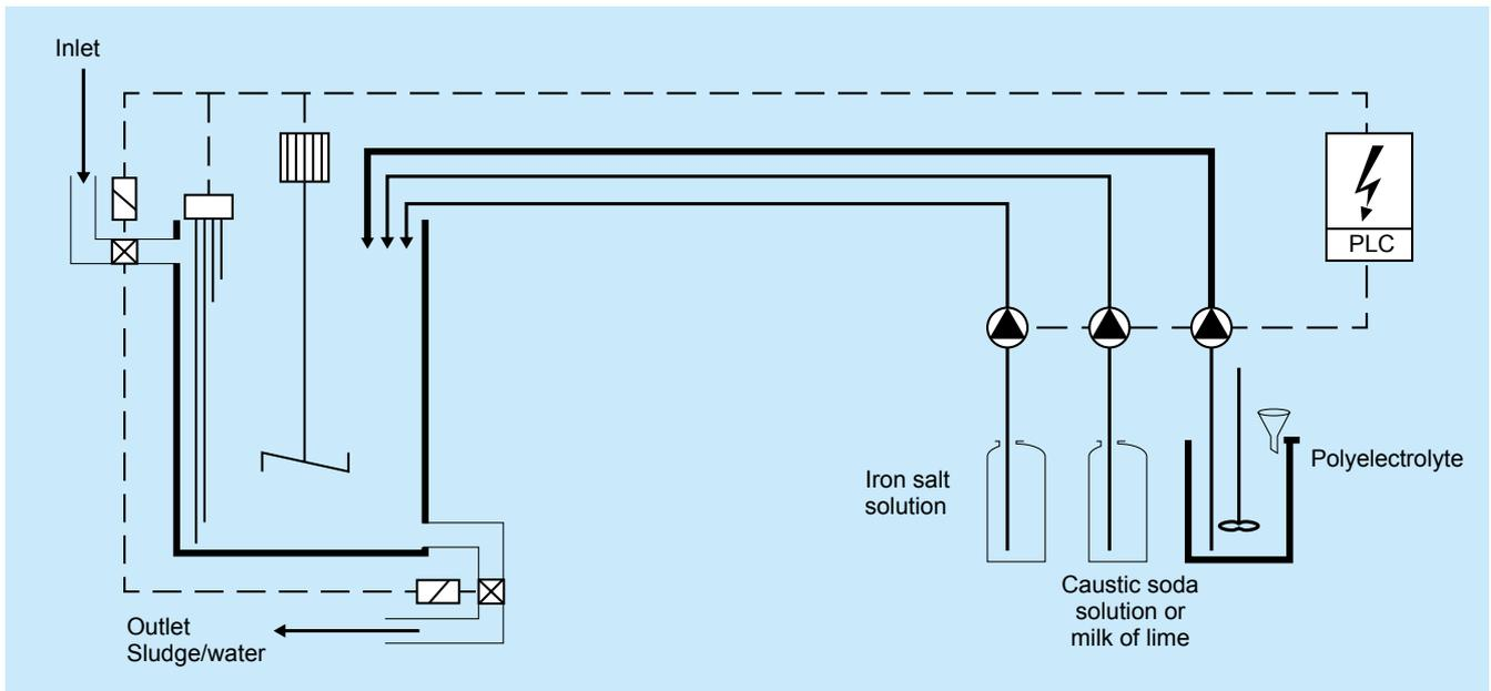
Fig. 3: Chemical-mechanical purification by precipitation and flocculation - batch process
