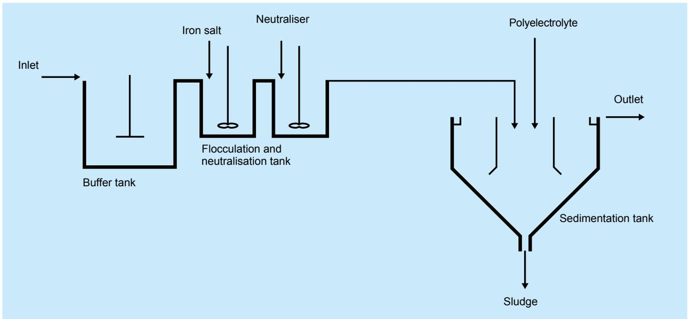
Fig. 2: Chemical-mechanical purification by precipitation and flocculation - continuous process
