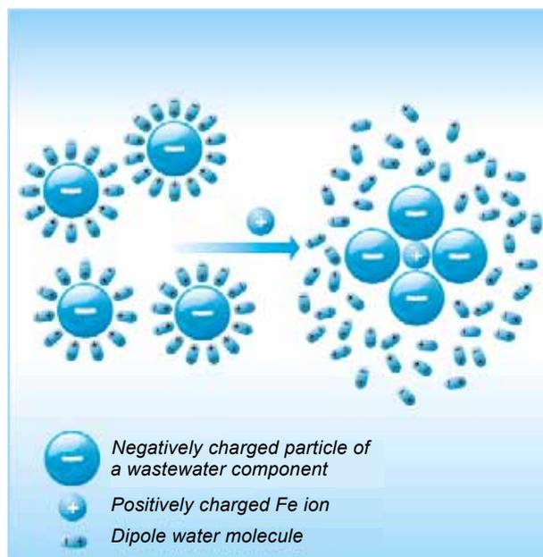
Fig. 1: Flocculation mechanism
